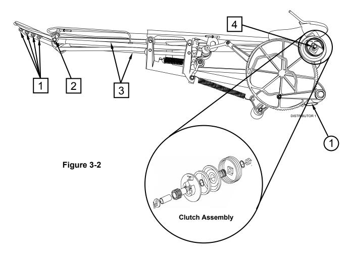
(1) Distributor support bearings (2 places): remove distributor and grease bearings once a year.
